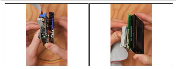
Stack the MakerShield onto the Wave Shield. Attach the LCD via ribbon cable, making sure it connects to the same pins at both ends. Connect the PIR sensor to the MakerShield via its included cable.
